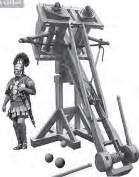
Rome ballista of 1/2 talent caliber
